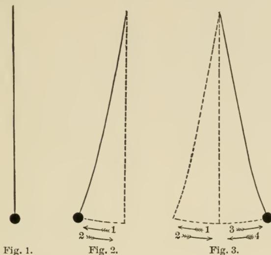
plumb line. Draw it aside and its weight will cause it to fall back again; this is a simple oscillation (Fig. 2). But our pendulum does not stop here; its motion continuing, it goes beyond its position of equilibrium, and then again falls back to it; this is a double oscillation (Fig. 3). And these movements back and forth will continue, so long as the impulse lasts which has been given to it.
